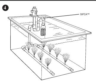
SIFCA<sup>TM</sup> is ideal in cases where pipe is connected to **Flo King** pump for special agitation effects (from bottom up, for instance, as shown above). Filter cartridges can be removed without disturbing pipe, pump, or tank components.
