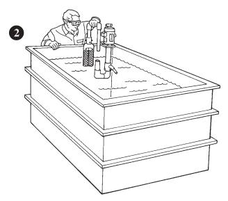
To change filters, just lift SIFCA<sup>TM</sup> and allow cartridges to drain in reservoir. Then install clean cartridges. While reattaching SIFCA to pump, move O-ring with thumb to reveal vent hole (see Illustration 3), releasing air from SIFCA<sup>TM</sup>. Now turn pump on and resume filtration.
