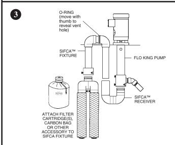
SIFCA<sup>TM</sup> assembles easily and can be used with standard **Flo King** accessories. *Receiver* can be mounted to pump in any direction for preferred positioning in tank. For filter or carbon changes, simply lift *fixture* and separate from *receiver*.
